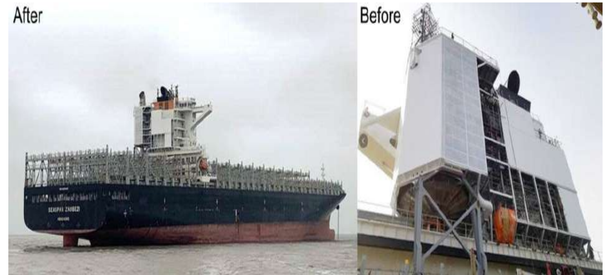
(Above left) Retrofitted 10,000 TEU vessel with added scrubber with perforated plate at port.
